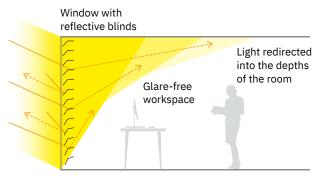
The upper section of the blinds directs the light into the depth of the room. The lower section enables glare-free light redirection to the ceiling.
